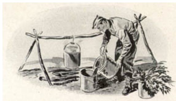
FIGURE 35. — Green vegetation being boiled in 5-gallon cans to make adhesive.
